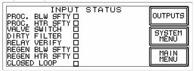
This screen allows the operator to view the status of the variables contributing to the input of material into the drying system. It also is useful in troubleshooting system issues (i.e. a dirty filter or low material level in a hopper).
